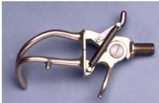
The Otto Bock Standard Two-Load Hook A flick of the small lever (usually done by brushing against the leg) lets you select between two different pinch forces
